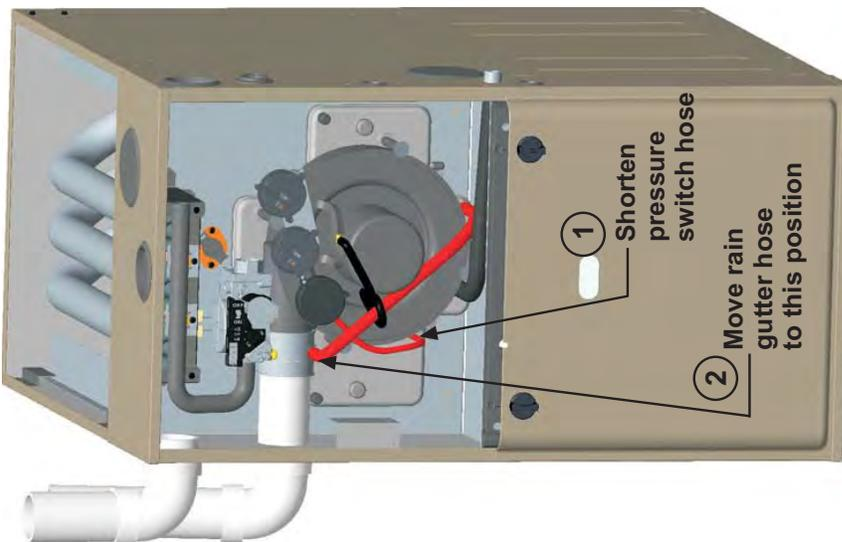
INDUCER ROTATED FOR LEFT SIDE VENTING
