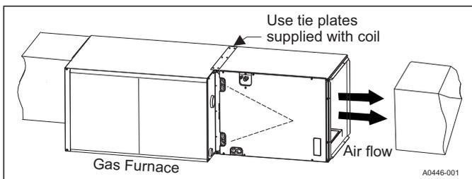
FIGURE 7: Horizontal Left or Right Application (Right Shown)
