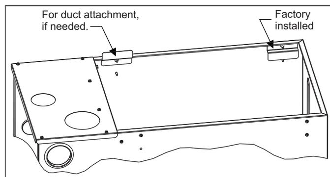
FIGURE 1: Duct Attachment
