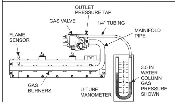
FIGURE 38: Reading Gas Pressure
