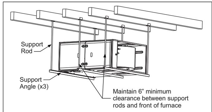
FIGURE 11: Typical Suspended Furnace / Crawl Space Installation
